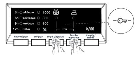
If pressed any button while child lock is active, the Additional Function Leds will blink on the display.
