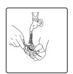
• After cleaning the filter, fit the filter cover and tighten it by rotating it in clockwise direction.
