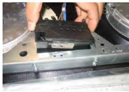
Pull the wiring sockets off terminal box
