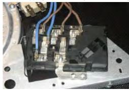
Take the wiring terminals off the heating elements
