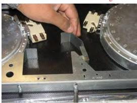
Take the wiring terminals off the heating elements
