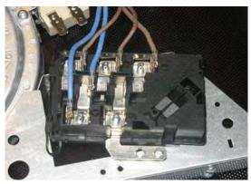
Remove terminal box heat insulating cover
