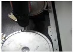
Unscrew ( t type ) heating element assembly springs they are screwed according to the matching numbers on heater&frame
