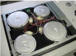
Loosen the silicone cable – to release the wiring harness
