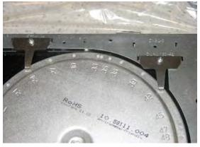
Remove (t type) heating element assembly springs from the hob frame
