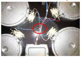
Unscrew terminal box and remove.
