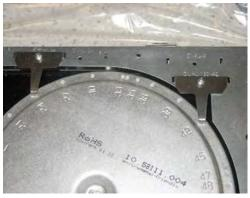
Remove ( t type )heating element assembly springs from the hob frame
