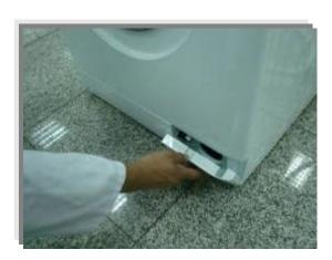
Remove the screw fixing the kickplate.
