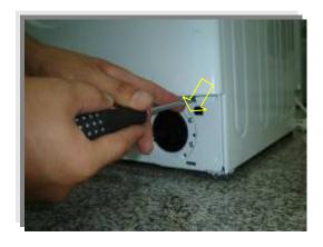
Remove two screws fixing the door lock.
