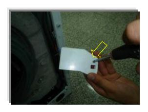
Remove the wire that is connected to the door lock.
