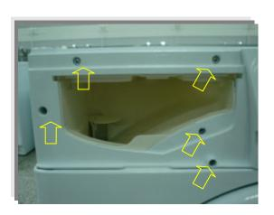
Remove two screws fixing the control panel.
