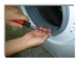
Remove the gasket-body fixing spring.
