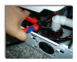
Remove pipe clip fixing the tub outlet hose.
