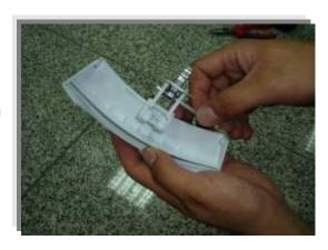
Remove the door handle spring as it is shown in the picture.
