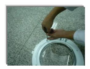
Remove the door inside plastic as it is shown in the picture.
