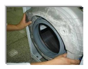
Hold the gasket and gasket-body fixing spring together, and pull them up.
