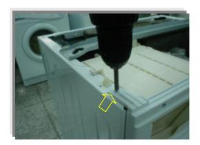
Remove one screw fixing the detergent box group.
