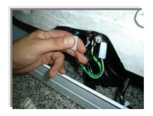
Remove one nut fixing the heater.
