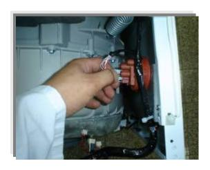
Remove the pressure switch as it is shown in the picture.
