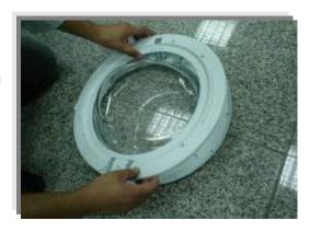
Remove the door hinge as it is shown in the picture.
