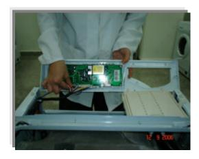
Remove four screws fixing the electronic card.
