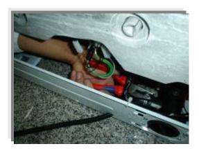
Remove the wire that is connected to the pump motor.
