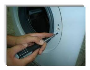
Push it down and remove the front panel.
