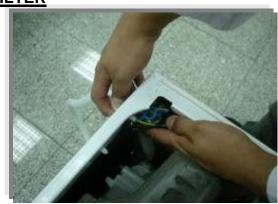
Remove the power cable group as it is shown In the picture.
