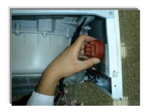
Remove the pressure switch hose handcuffs And pressure switch hose as it is shown in the picture.
