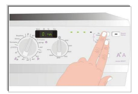
Wash, rinse and spin LEDs will flash for 2 seconds, if any button is pressed on the control panel.
