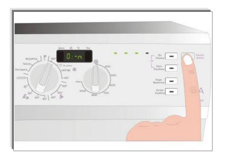
Press the first and second function button for 3-4 seconds to inactivate child lock.
