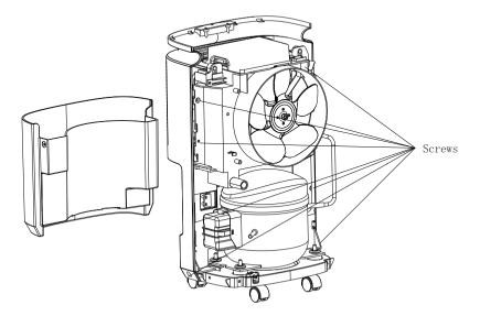
4. Remove the front cover according to the picture's direction.
